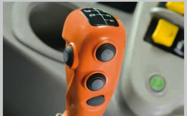
Comfort clutch and Powershift. Simply change gear at the push of a button without pressing the clutch.
