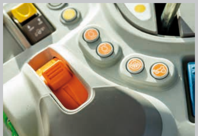
New: two engine speed settings. Pre-programmed efficiency for routine operations. (5125 Only)
