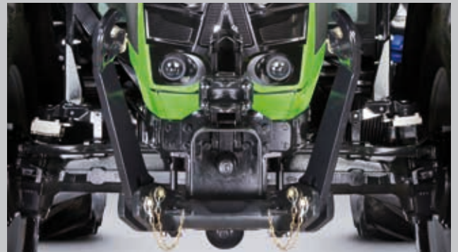
Front lift and PTO. Lifting capacity of 2,100 kg and 1,000 PTO (indent only).
