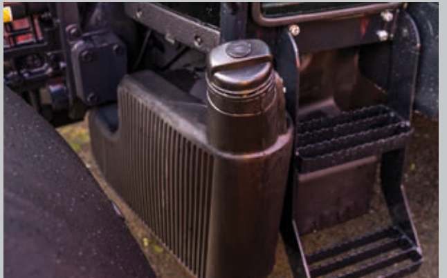
A fuel tank that holds up to 150 litres and allows long working periods (depending on model).
