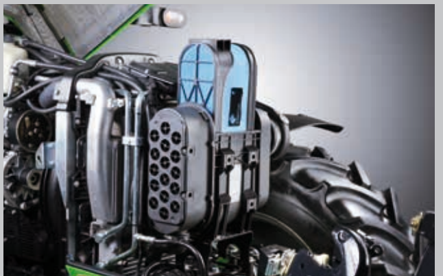
The PowerCore air filter supports engine efficiency ...
