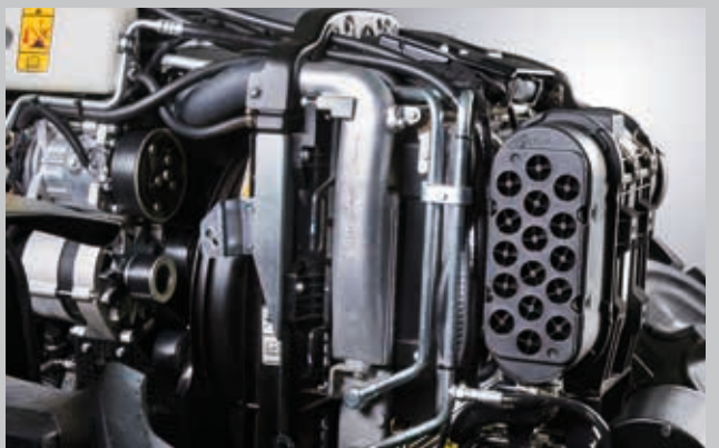
... as does the easy-to-clean cooling system with optional viscous fan.
